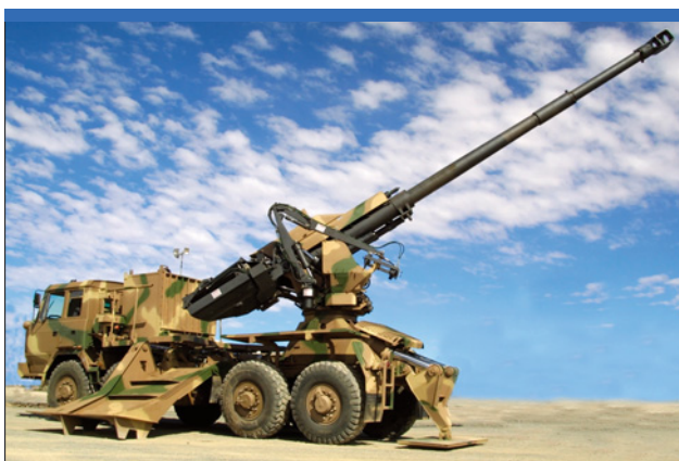
The Condor mounts the ordnance of Denel's G5-2000 towed artillery system on the Tatra 8 x 8 chassis, which is produced under license by India's Bharat Earth Movers. (Denel)
