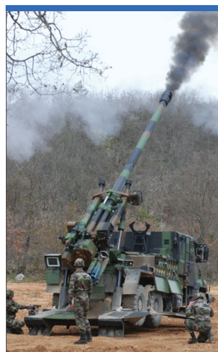
The most recent version of the Caesar, seen here during trials in April 2007, is based on a Renault chassis. It is the definitive version for the French Army. (Nexter)
