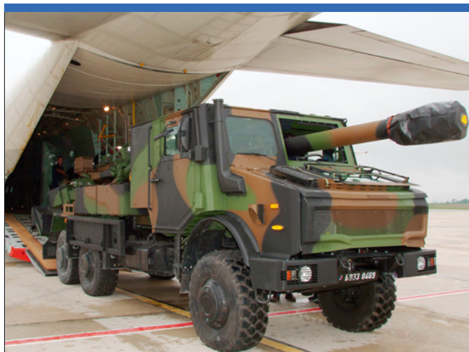
Nexter's Caesar 155-mm/52-calibre self-propelled artillery system can fire extended range full-bore - base bleed (ERFB-BB) projectiles to a maximum range of 42 km. This is the Unimog-based version seen rolling out of a Hercules. (Nexter)
