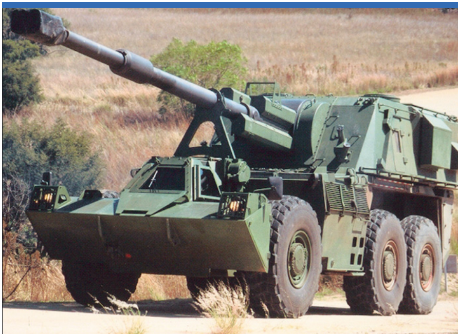
The G6-52 has a maximum speed of 80 km/h on roads and an operating range of 700 km. Air transportability was not a significant consideration in the design of the G6-52, which has a combat weigh of 49,000 kg. (Denel)
