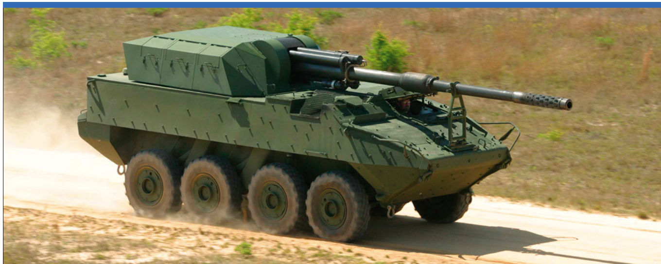
This demonstrator combines a Denel 105 Leo (originally developed as a towed gun) and a General Dynamics LAV III. (Denel)
