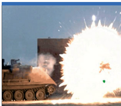
The Israel Military Industries hard-kill Iron Fist is competing in Israel against the Rafael system Trophy, but is claimed to be lighter and thus adaptable to smaller vehicles. Like Saab's solution, it appears to use blast effect to crush the incoming warhead rather than detonate it or achieve a direct hit-to-kill. (Israel Military Industries)
