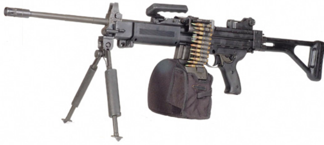
The 5.56 mm Negev LMG was developed by Israel Weapon Industries to meet the demands of the Israel Defense Force. The standard Negev with 200-round 'soft assault drum' is shown here. (IWI)
