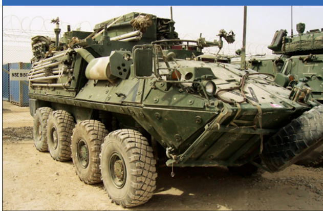
One GD Canada-built derivative of the Mowag Piranha is the Canadian Forces' Bison, with IBD Mexas and Amap-1 for protection against small arms fire, mines and IEDs. (Canadian Forces)
