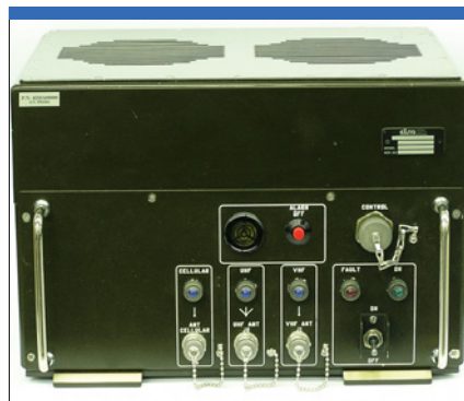
Developed to meet the needs of the Israel Defence Force Elisa's Electronic Jammer Against Bombs (Ejab) has been in Polish Army vehicles operating in Iraq. The modular system can be either hand-held or vehicle mounted. (Elisa)
