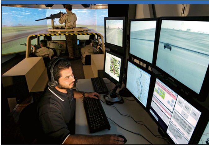
Mounted in two standard 53-foot trailers the Virtual Combat Convoy Trainer, such as the Lockheed Martin Simulation and Training Systems design shown here, can be moved to different locations to support training. (Lockheed Martin)
