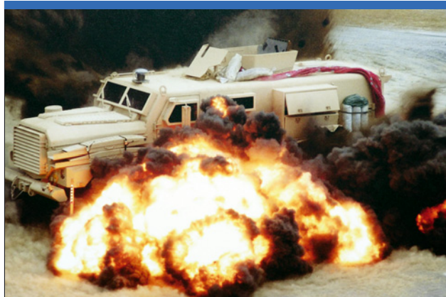
A Force Protection 6 x 6 Cougar Joint EOD Rapid Response Vehicle undergoes the first of a four-shot series of explosions at the US Army's Aberdeen Test Center. The US plans to use more Mrap vehicles such as this in the patrol and convoy escort roles. (US Department of Defense)
