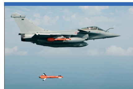
Shown on a Dassault Rafale, the Sagem AASM will replace laser-guided bombs and the AS.30L missile in French service. It is already cleared on the Mirage 2000. (Dassault Aviation)
