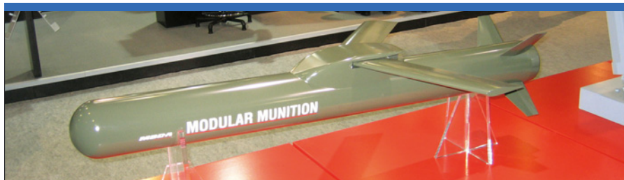
The MCT will probably serve as a basis for the development of the new EMM family of anti-armour and anti-structure weapons. This is the MBDA air-launched variant of the planned MCT. (Armada/EHB)
