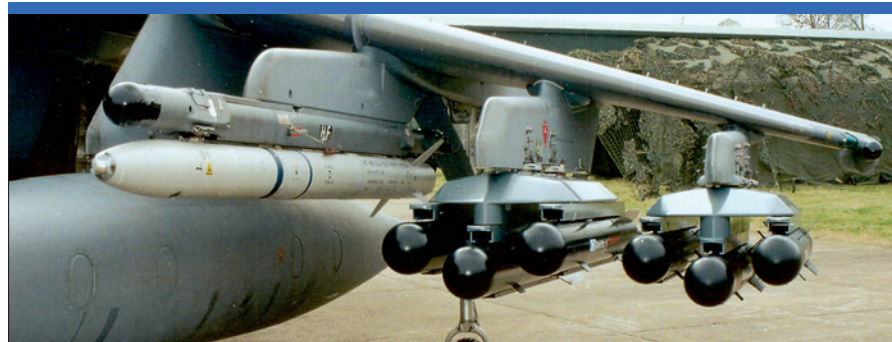
The MBDA Brimstone anti-armour missile is shown on triple racks under the wing of a British RAF Harrier GR9, with the same company's AIM-132 Asraam mounted inboard. (MBDA)
