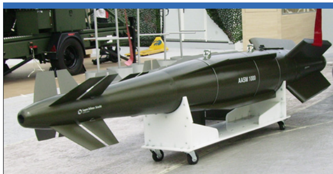
At the recent Paris Air Show, Sagem revealed a new family of Aasm missiles, like this 1000-kg weapon, to complement the current 250-kg Aasm. The other members use 125 and 500-kg bombs. (Armada/EHB)
