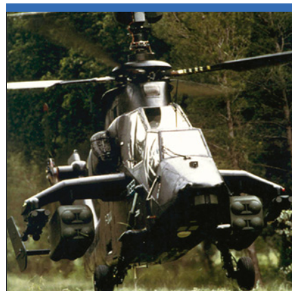
German Army Eurocopter Tigers will replace the MBDA Hot 3 anti-armour missile with the same company's Pars-3 LR, shown here in wing-mounted four-round pods. (MBDA)
