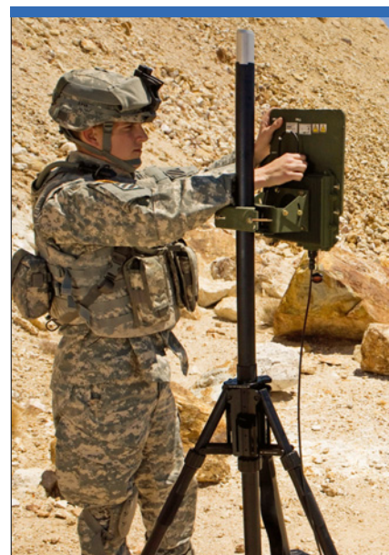
Harris has recently unveiled its high-speed broadband Ethernet radio, the 7800W, which transfers IP traffic out to 50 km under clear line-of-sight in a fixed point-to-point configuration. The 2.3-kg radio transmits 70 Mbps in secure mode through its 256-bit AES encryption. (Harris)
