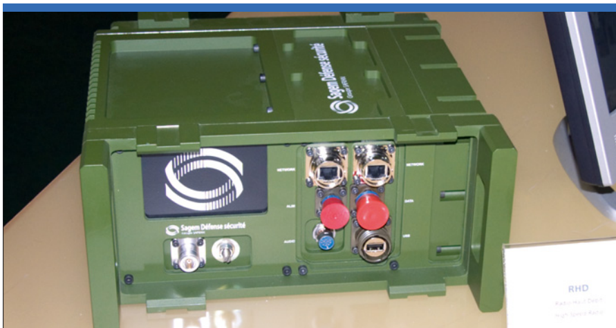
In 2006 Sagem introduced its RHD high data-rate radio, which is optimised for the high-electronic warfare urban environment. The RHD, which offers four Mbps at full-duplex operation, was tested by France's Centre d'électronique de l'armement. (Armada/JK)
