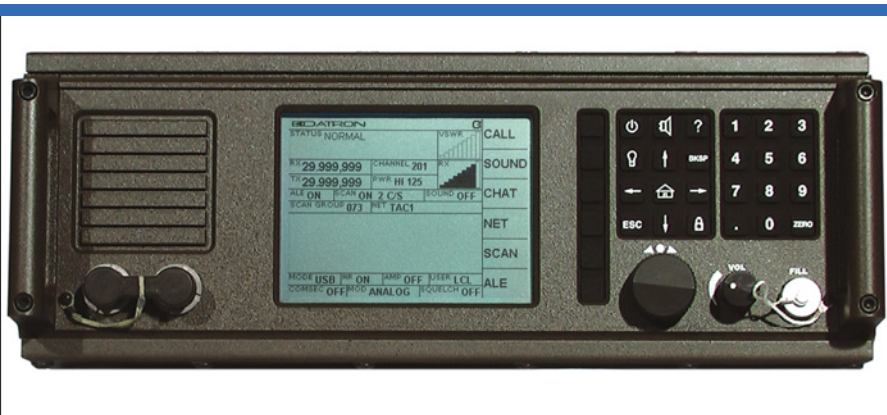
The RT7700 tactical HF software-defined radio from Datron provides AM, AME, LSB, ISB, USB, data and digital audio coupled with digital comsec over IP addressable channels and a 10/100BaseT Ethernet port. The radio can capture and transmit maps and tactical data, secure voice and e-mail transmission between 1.6 and 30 MHz. Shown is the RT7700 transceiver, capable of supplying over 125 watts (single sideband), which could be used in combination with a series of VHF feeder networks for long-haul transmission of prioritised data. (Datron)
