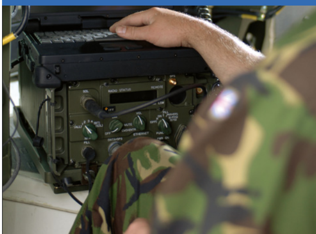
ITT's High Capacity Data Radio (HCDR) is the epitome of soldier-proof equipment. The radios autonomously form self-healing, ad hoc UHF networks configured by the user simply switching it on. . . . the radio does the rest. (ITT)
