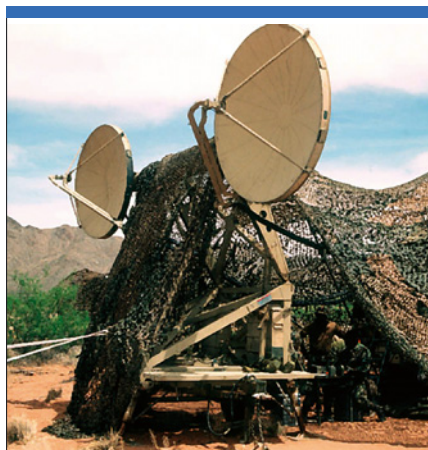
The US military has been using the troposcatter solution for years (as have many countries worldwide). Here is one US Army mobile solution, the dual 9.5-inch AN/TRC-170 troposcatter microwave dish assembly. Comtech Systems provides an upgrade to double the bandwidth from four to eight Mbps. (US Army)
