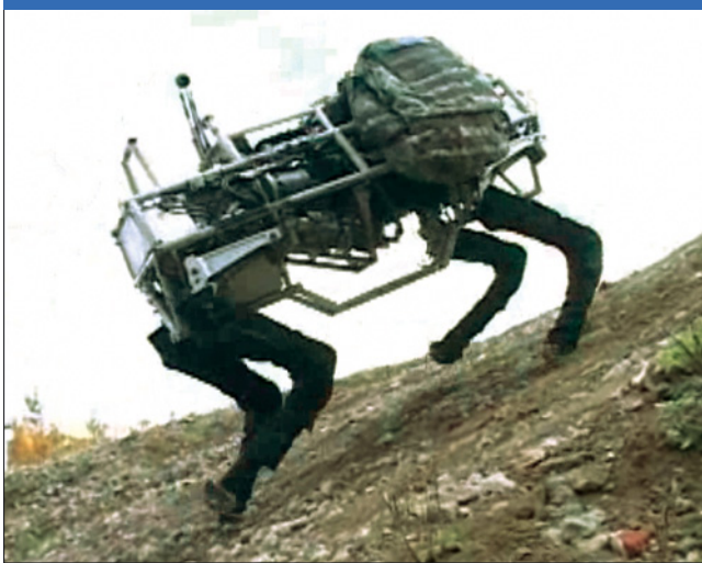
This photo is a low-resolution screen shot of the captivating Bigdog video that is available on the Boston Dynamics website (found at: bostondynamics.com ). Thus far in development the robotic pack mule has trotted along at around five km/h, climbed a 35° slope and carried a 55-kg load. (Boston Dynamics)
