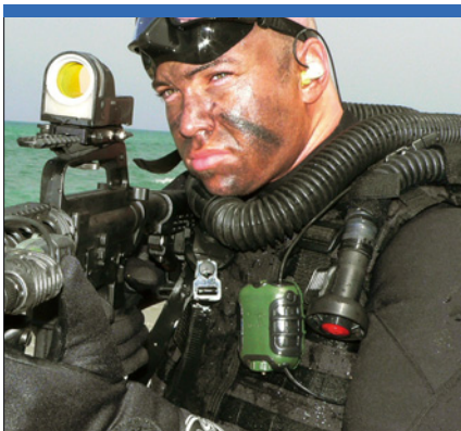
The Silyn Quiet Ops tactical communication headset and ear protector provides a passive and active noise attenuation system that lowers the level of high-decibel environments, such as that found in military aircraft or high-intensity impulse noise (e.g. weapon fire). (Silyn)
