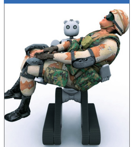
Scheduled for a 2008 release date the Bear from Vecna Robotics is being designed to safely transport human casualties out of dangerous combat and contaminated areas. The robot will have 20 joints, stand two metres tall and weigh around 100 kilos, not counting its, up to 181 kg, casualty load. (Vecna Robotics)
