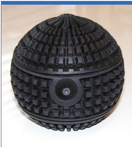
The Short Range Throwing Camera from Macroswiss is not a throw-away camera but a 'throw-to' remote observation system designed to broadcast a panoramic view of the surrounding area (in a room, over a wall, in a street, etc) to a remote operator. The self-righting ball transmits video information on the 2.4 GHz band, to 300 metres for up to five hours. (Macroswiss)
