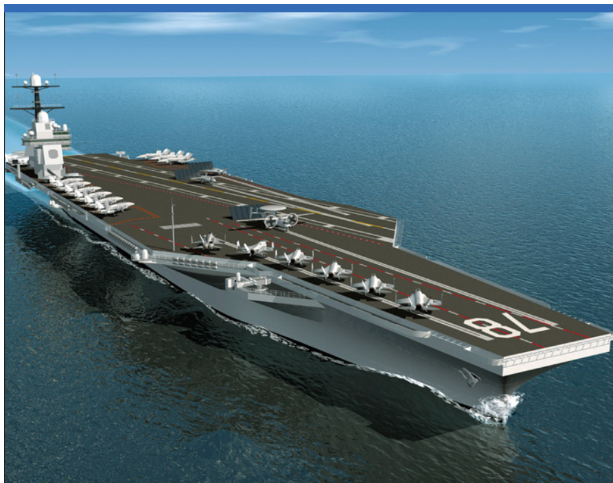
CVN 78 will be the first of the CVN 21 new generation US Navy carriers. It will be named after former President Gerald Ford. The most noticeable feature is the greatly reduced size of the island. (Newport News)
