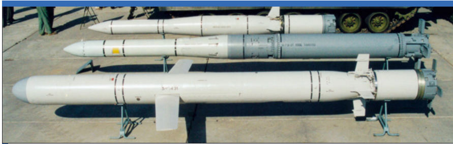
With the Club series, Novator offers an extensive range of anti-ship missiles with ship-launched (background), submarine-launched (centre) and air launched derivatives. The latest Club-M (not seen here) is a land-launched land-attack version, which has an air-defence avoidance capability. (Armada/YL)
