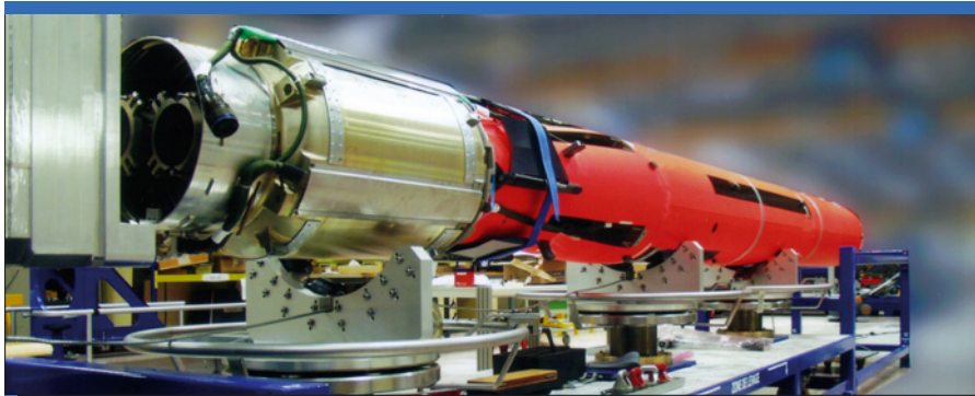
In the context of the Franco-Italian Fremm frigate programme, MBDA is developing a ship-launched derivative of the air-launched land-attack Scalp missile. While retaining most of its innards, the missile, known as the Scalp Naval, is totally repackaged to fit in vertical launchers. (MBDA)
