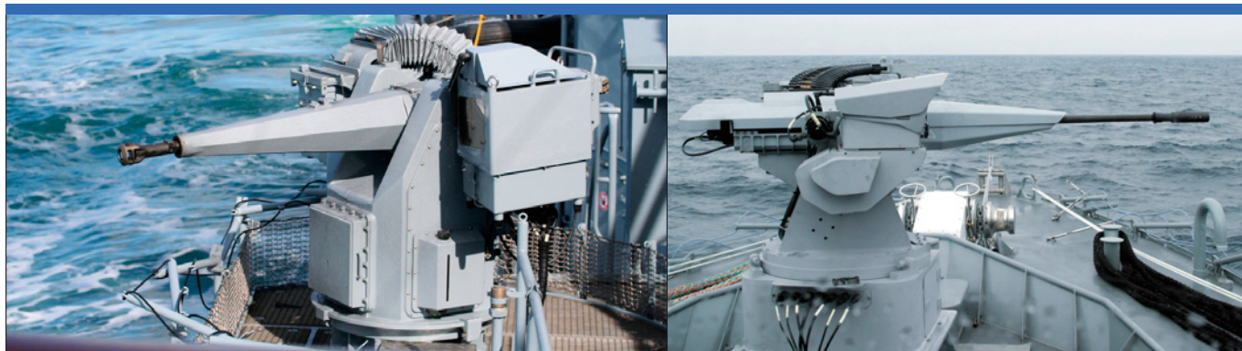
Remotely operated guns, such as the Rheinmetall MGL and Nexter-DCNS Narwhal mounts, were not taken too seriously when they were introduced or being developed a few years ago. However, due to their ease of installation (deck-penetration free) and the fragmentation rounds they fire in conjunction with high-performance optical trackers, they are likely to represent valuable assets for the protection of not only corvettes, but also humanitarian support ships in waters infested with pirate boats. (Rheinmetall and Nexter)
