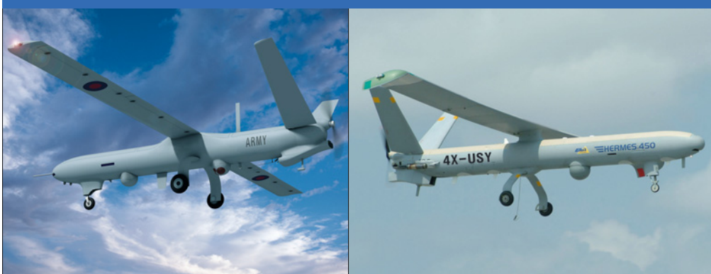
There are notable differences between the new Hermes 450-based Watchkeeper (seen on left as a montage involving a mock-up) and the original drone developed by Elbit. Not only does the Watchkeeper have two payload bays, it has a faired wing root and nose wheel strut. The engine radiator scoop also seems to have received attention, but one may legitimately wonder whether the sensor under that scoop will remain there. (Thales)
